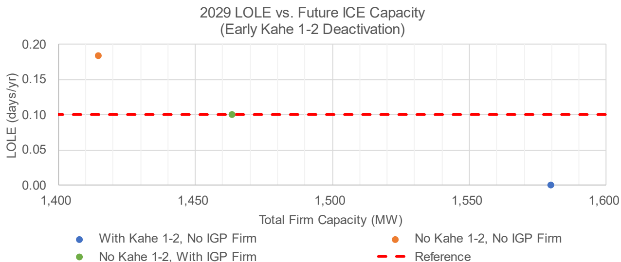
Figure 2-32: O’ahu LOLE vs. future firm in 2029 with early Kahe 1-2 deactivation. Deactivation schedule sensitivity.
