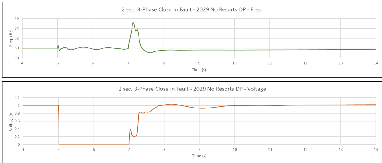
Figure 78 Dynamic stability simulation results, Lānaʻi no resort scenario resource plan, year 2029, three-phase close in fault
