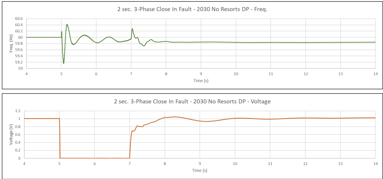
Figure 81 Dynamic stability simulation results, Lānaʻi no resort scenario resource plan, year 2030, three-phase close in fault
