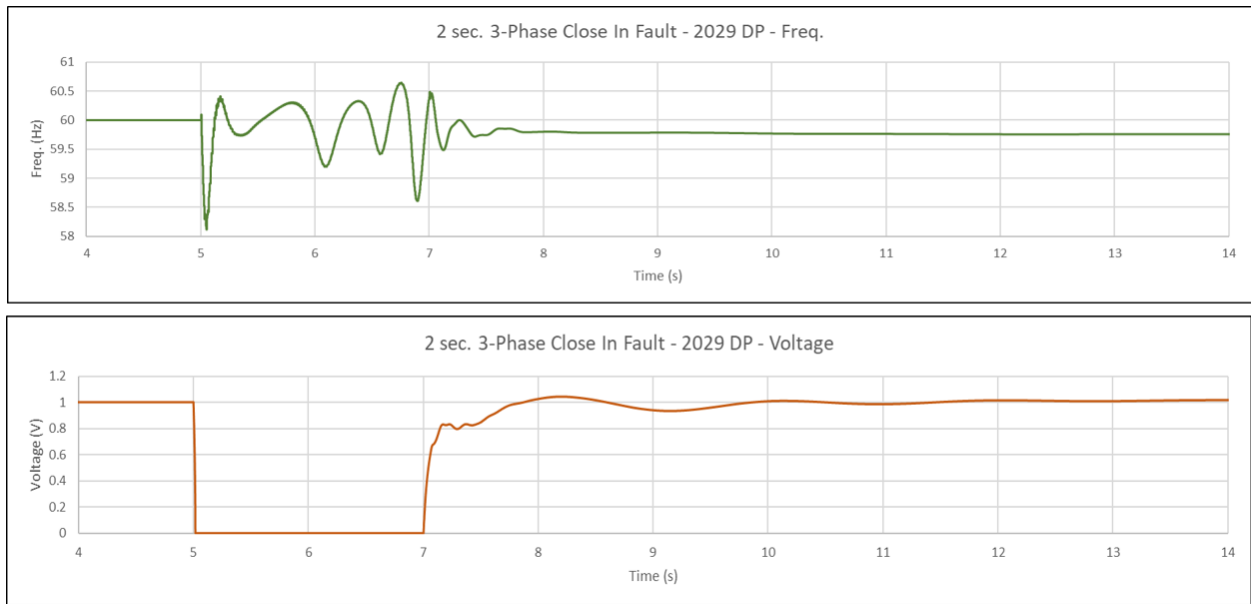
Figure 72 Dynamic stability simulation results, Lana'i base scenario resource plan, year 2029, three-phase close in fault
