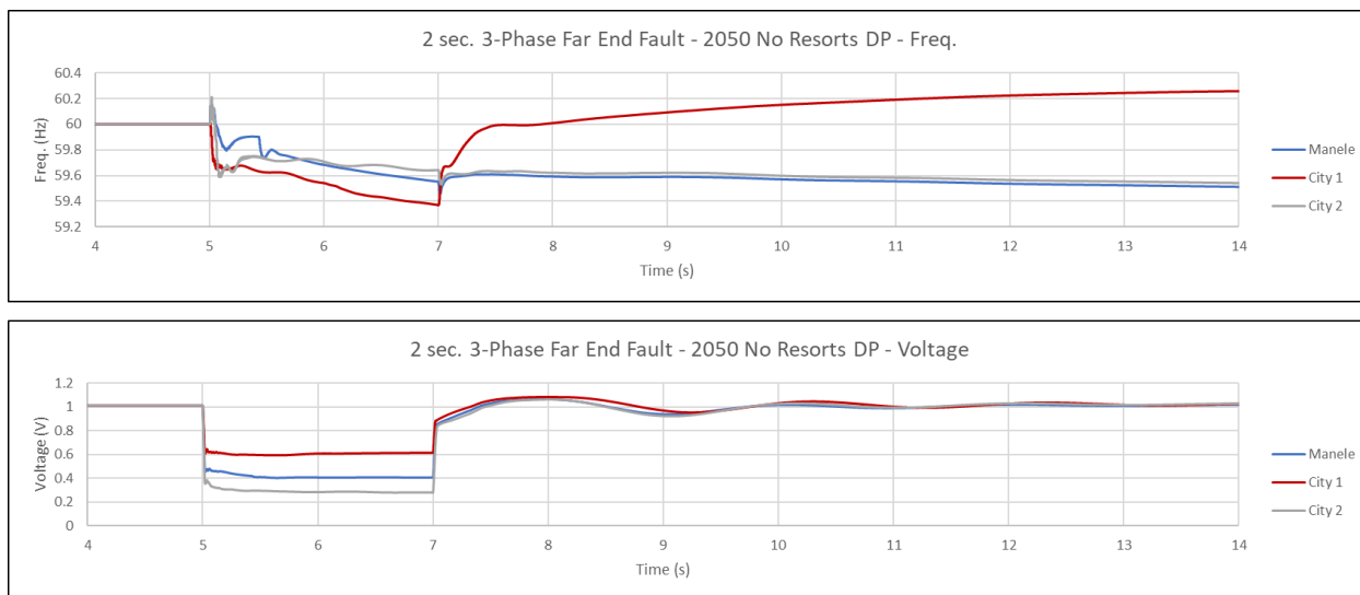
Figure 85 Dynamic stability simulation results, Lana'i no resort scenario resource plan, year 2050, three-phase close in fault
