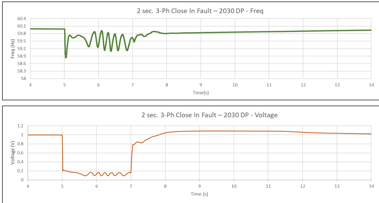
Figure 66 Dynamic stability simulation results, Moloka'i base scenario resource plan, year 2030, three-phase close in fault
