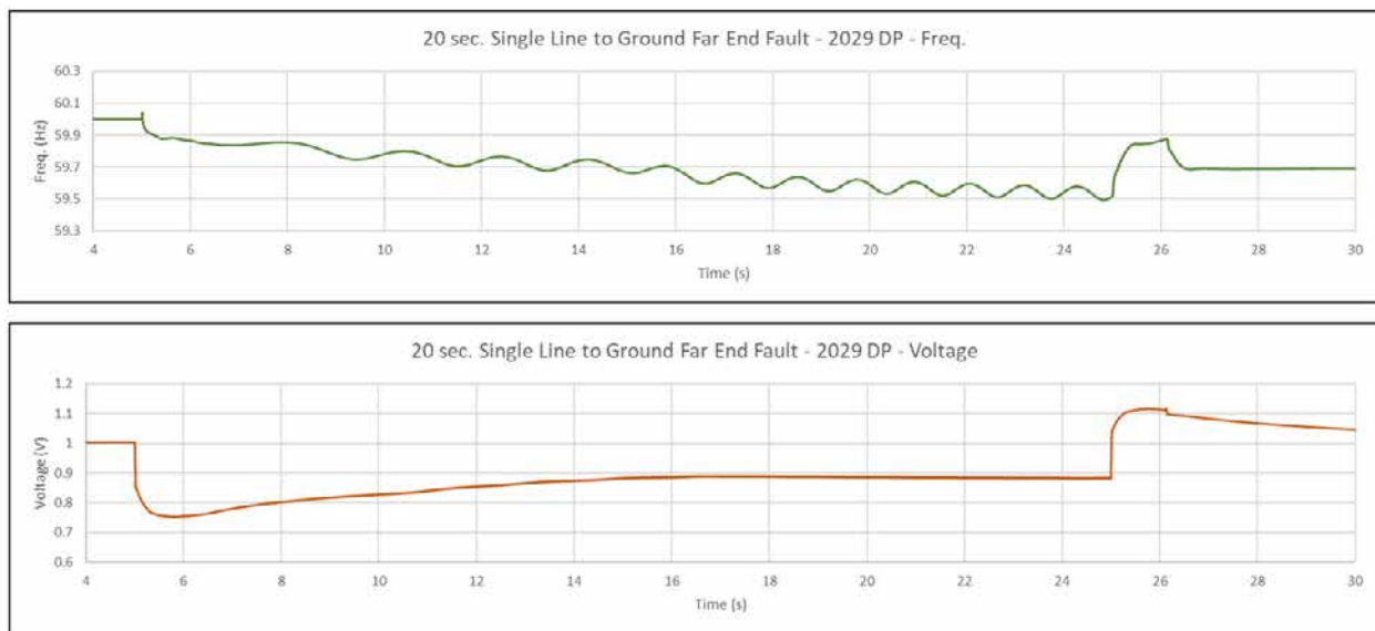
Figure 74 Dynamic stability simulation results, Lana'i base scenario resource plan, year 2029, single phase far end fault with high fault impedance
