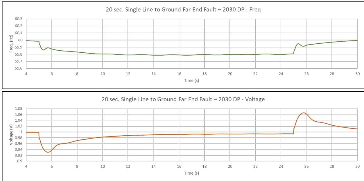
Figure 68 Dynamic stability simulation results, Moloka’i base scenario resource plan, year 2030, high impedance far end fault
